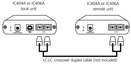
Maximum 500 m multimode fiber for IC404A; maximum 10 km single-mode fiber for IC406A
