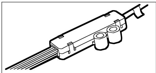
Terminate loose tube cables at fibre cross-connects.
