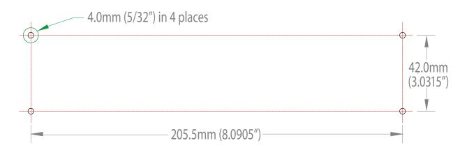
FIGURE 4-3. DIRECT SURFACE MOUNTING MEASUREMENT STENCIL
