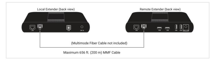
STEP 2. Connect the Local Extender to the computer's USB 3 port using the included USB cable.
