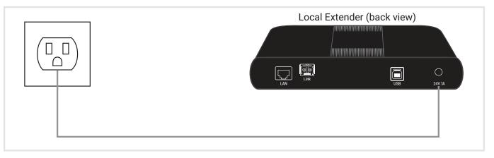
STEP 4. Power the Remote Extender with the included 24 V, 2.71 A AC adapter and tighten the locking ring.
